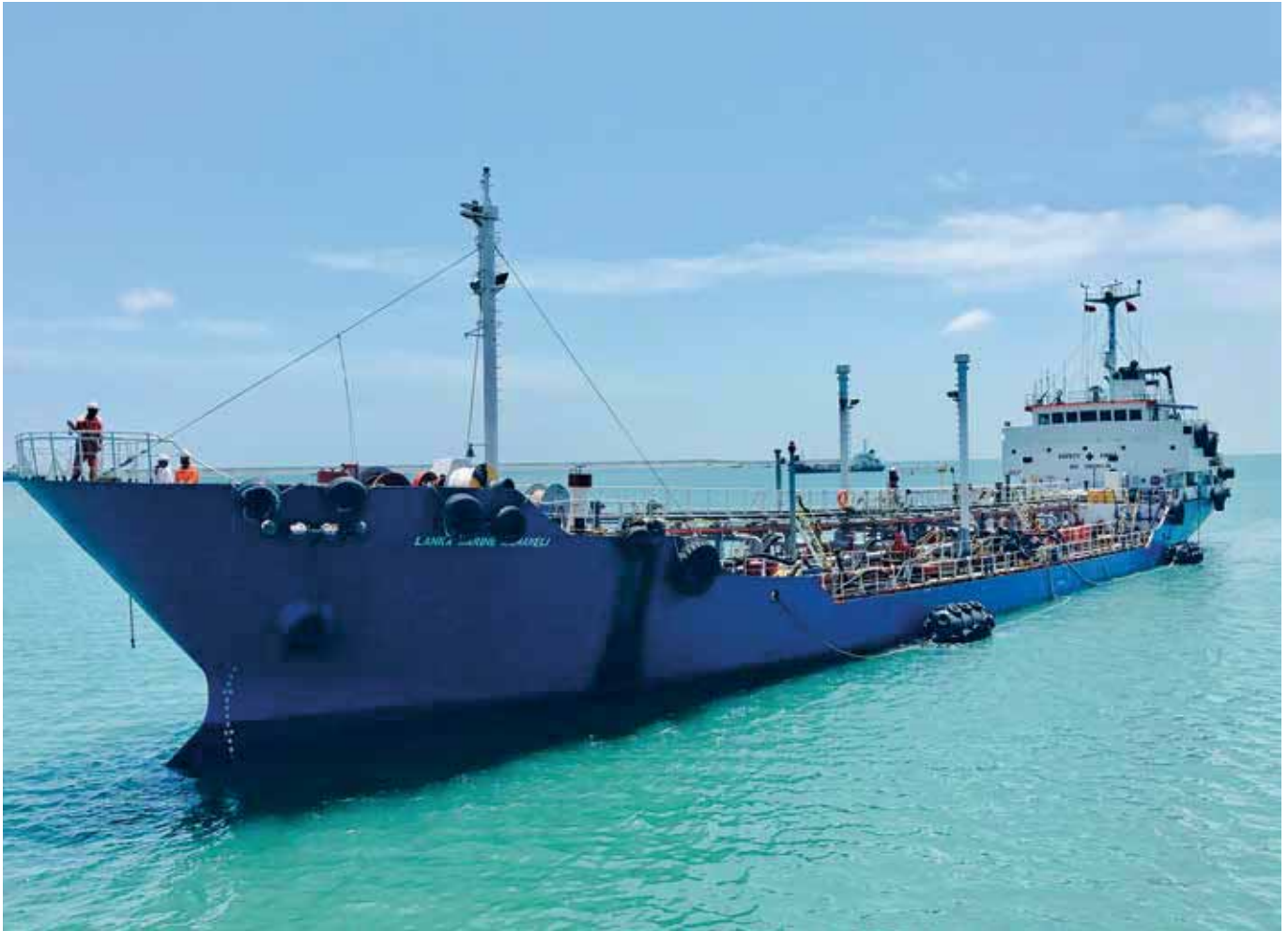
The "MT LM Mahaweli", Sri Lanka's first double hulled, double bottomed bunker barge commissioned by LMS
